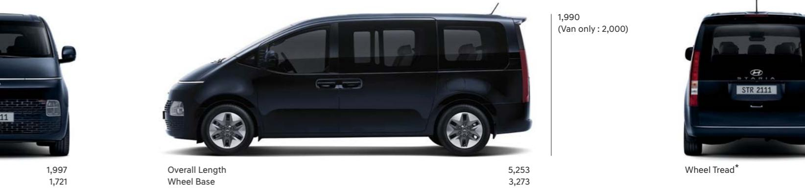
Unit : mm \*Wheel tread • 18" wheel (front/rear) : 1,721/1,732 • 17" wheel (front/rear) : 1,732/1,743 • 17" wheel for van only (front/rear) : 1,732/1,716
